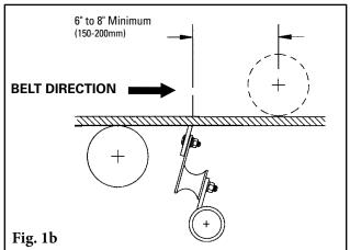
**1. Select best location:** Find location either in front or behind the belt cleaner 6" to 8" (150-200mm) (Fig. 1a and 1b). Also keep 6" to 8" (150-200mm) away from return rollers.
