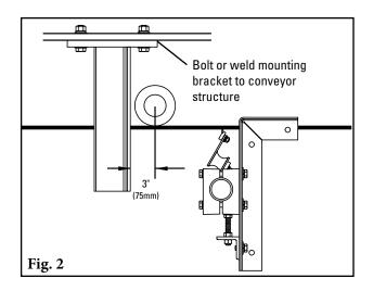
2. Locate the position for the mounting brackets. The position of the mounting brackets can vary slightly depending on the diameter of the live-shaft hold-down roller. As a rule of thumb, position the front of the mounting bracket 3" (75mm) past the contact point where the roller will meet the belt (Fig 2). Ensure there is enough length in the bracket slot to allow the roller to flatten the belt. Use C-Clamps to hold the brackets in place, then bolt or weld to structure.
